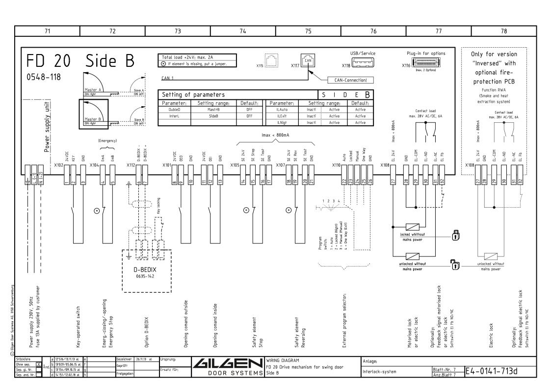
2 4 8 Optional relay PCB for FD 20 **JILJEN** Notes description DOOR SYSTEMS Gilgen Door Systems AG Freiburgstrasse 34 3150 Schwarzenburg Diagram drawn: door is closed; mains off \* If element is missing, put a jumper. (1) If element is missing, put a resistor. a 12'551/20.01.14 al Gezeichnet 13.06.13 al Ursprung: WIRING DIAGRAM Anlage: Optional relay PCB for FD 20 Ersatz für: E4-0141-715a DOOR SYSTEMS 0548-215
